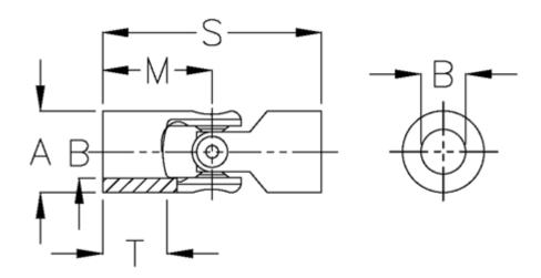
$\begin{array}{lll} A & = 50 \\ B \ H7 & = 32 \\ M & = 66 \\ MD \ max \ N \ m = 120 \\ s & = 132 \\ T & = 40 \\ \end{array}$
